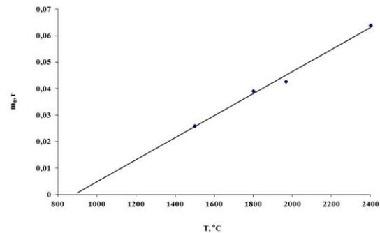
*Fig. 2. Maximum weight gain as a function of nitridation temperature for the exponential stage of the process.*
